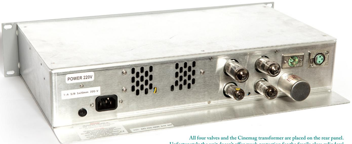
All four valves and the Cinemag transformer are placed on the rear panel. Unfortunately the unit doesn't offer much protection for the fragile glass cylinders!
